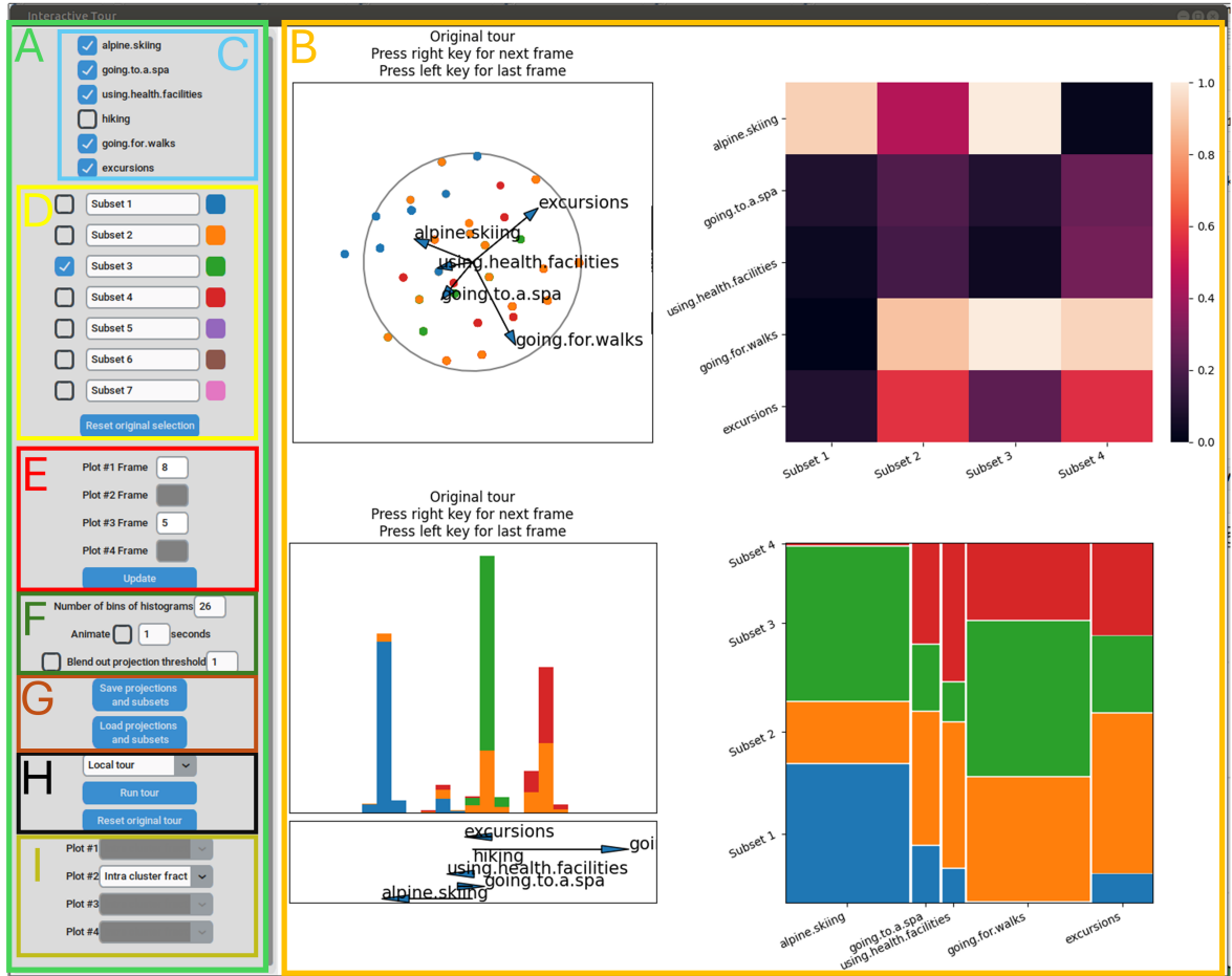
Figure 4: Overview of the GUI. A: Sidebar controls; B: Display area; C: Feature selection checkboxes; D: Subset selection with color indicators; E: Frame selection interface; F: Interfaces for adjusting the number of bins of histograms, animating tours and blending out projection axes with a low norm; G: Save and load buttons; H: Interface for starting new tours; I: Metric selection interface.
